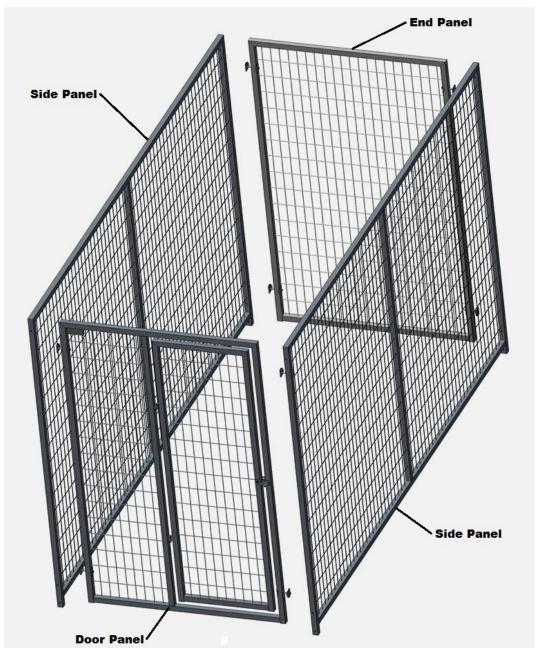
The door panels and end panels are always installed in between the two side panels. Since the doors both open in and out the door panel can also be installed with the door on the left or right. Side Panels have the 2" legs, end panels do not.
