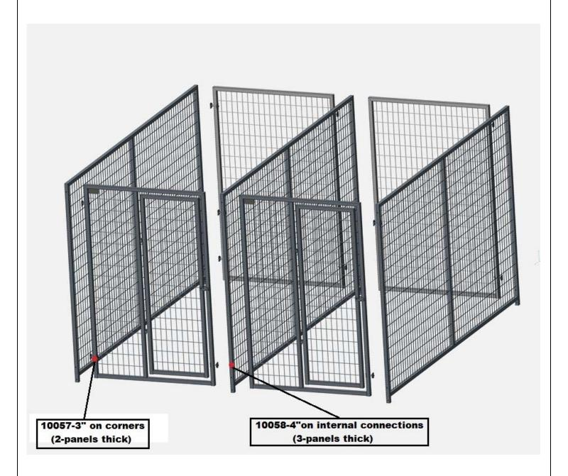
Use our 10057 - 3" bolt assemblies on all outside corner connections or wherever only two panel thicknesses are connected.
