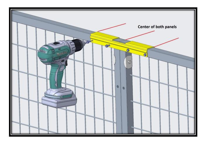
2) For bottom coupling, slide the 10655 coupling around both mating panel legs and center the couplings rectangular hole around the legs, you may need to tap it on with rubber mallet to push it over some welds. Once fully seated and centered the panels install the 8 stainless steel self-drilling screws with a drill and 5/16" hex head bit.
